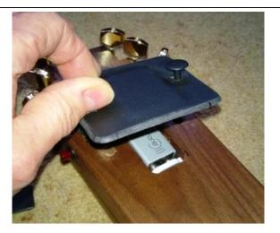
Remove the plastic pins and pull away cover.
